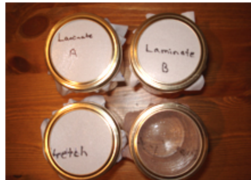
Figure 3. Materials stretched over mason jars and held in place by metal screw ring.
