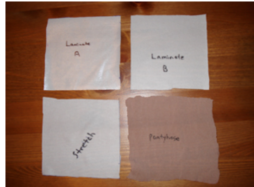
Figure 2. Materials to be tested cut into 10cm x 10cm squares.
